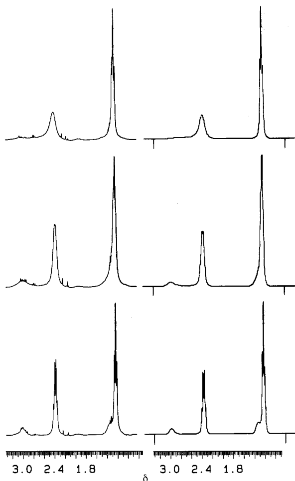
Fig. 1 Experimental (left) and calculated (right) 1 H NMR spectra of [Pd(EtCN) 4 ] 2+ 2 and free EtCN. c M = 57.2 mmol kg –1 , [L] = 1.031 mol kg –1 , T = 301.5 K, T 2 * = 0.6 s, τ C –1 = 63.1 s –1 (bottom); T = 316.3 K, T 2 * = 0.5 s, τ C –1 = 135 s –1 (middle); T = 336.4 K, T 2 * = 0.7 s, τ C –1 = 271 s –1 (top)
